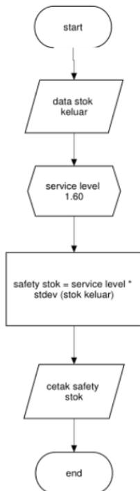
Gambar 4. Flowchart Hitung Safety Stock
