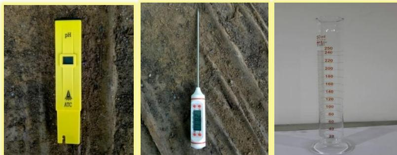
**Gambar 9.** Alat pengukur PH (PH-meter), pengukur suhu (termometer) dan pegukur Volume (gelas ukur)
