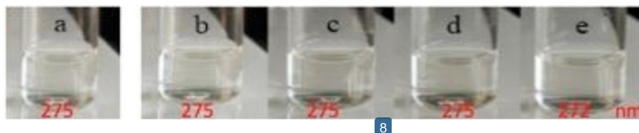
Fig. 2. Photos of NBP under various temperatures: at room temperature (a), 303 K (b), 313 K(c), 323 K(d) and 333 K (e). The UV absorbance maximum of each sample is showed in the lower series
