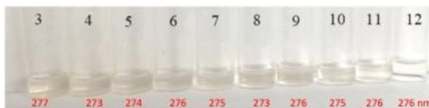
Fig. 1. Photos of NBP under various pH ranges (from pH 3 to pH 12). The UV absorbance maximum of each sample is showed in the lower series
