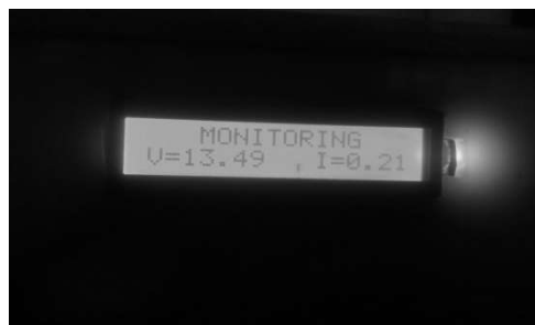
Fig 4.4 Testing voltage and current sensors with load
