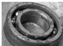
Figure 2. A Bearing fault caused by corrosion
