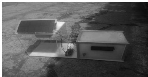
Fig 4.2 Testing of solar cell voltage
