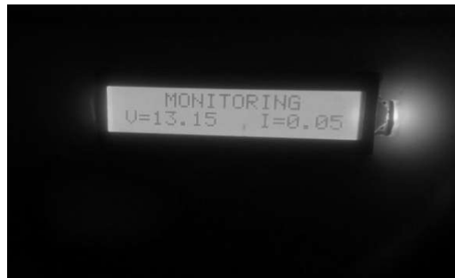
Fig 4.3 Testing voltage and current sensors with no load
