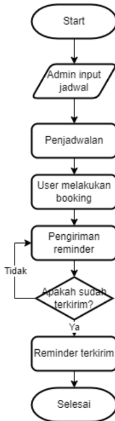
Gambar 3.3 Flowchart Reminder Otomatis
