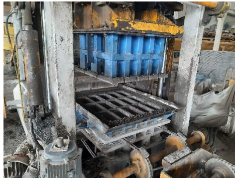
Gambar 3.14 Block Moulding dan Hydraulic Pressure
