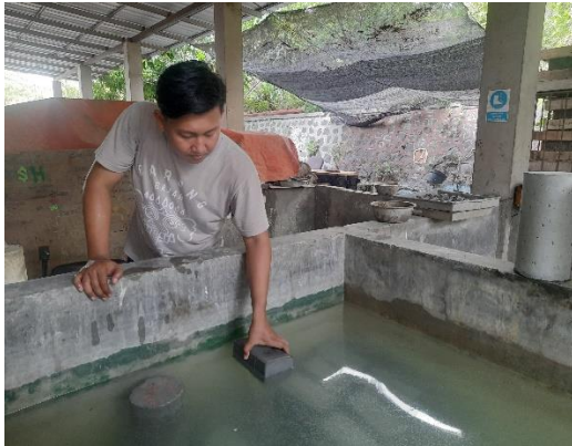
Gambar 85. Proses Perendaman Paving Block
