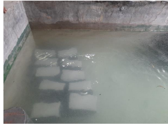
Gambar 86. Perendaman Paving Block Selama 24 Jam
