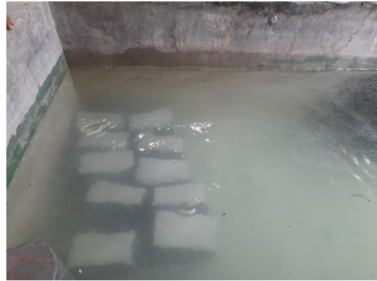
Gambar 86. Perendaman Paving Block Selama 24 Jam
