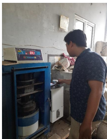
Gambar 84. Proses Pengujian Kuat Tekan Paving Block
