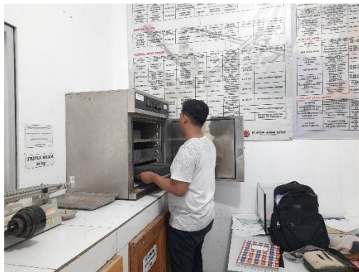
Gambar 87. Proses Pengovenan Paving Block
