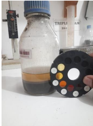
Gambar 4.12 Hasil Uji Kebersihan Pasir Terhadap Kadar Organik
