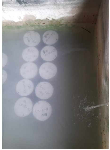
Proses Curing Benda Uji
