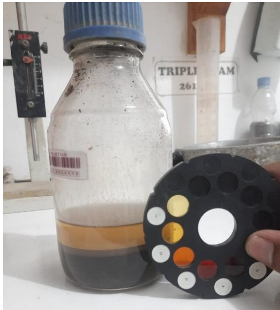
Pengujian Kadar Organik Pasir
