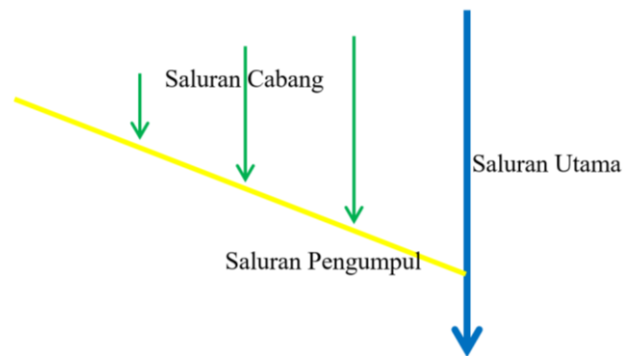
Gambar 2.3 Jaringan Drainase Grid Iron
