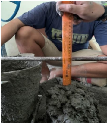
Gambar 3. Hasil slump Test
